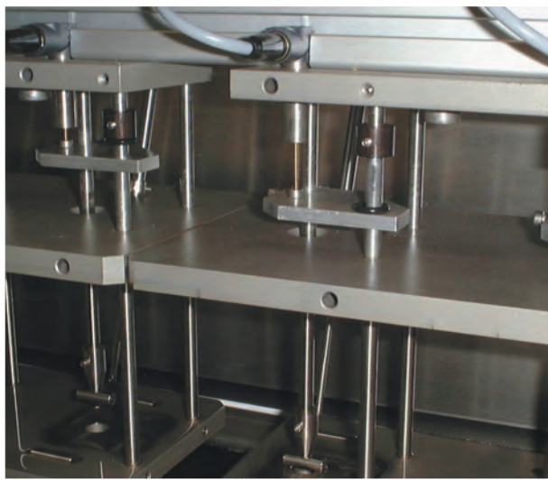
Measuring head: this contains the temperature measuring device and the position sensor.
