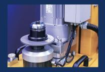
It enables precise measurement of torque for ground penetration.
